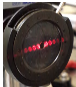
Figure 5: Resultant pattern of 2mm beam on iris after reflecting off the MEMS Grating Modulator
