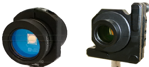
Figure 3: MEMS Grating Modulator in Slip Ring (left) and Gimbal Mount (right)
